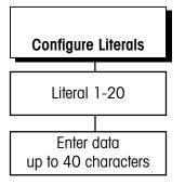
Literals are text strings such as site name or address that can be printed in a template. They can be up to 40 characters in length and are referenced by a field code. See the section entitled Configure Template Sub-block in this chapter. You can program up to 20 literals. To configure literals:
