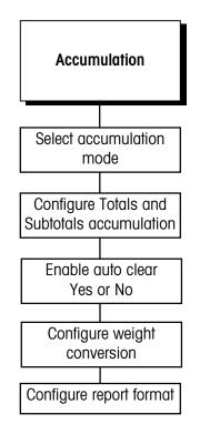
The LYNX terminal uses the primary weight unit (calibration unit) for accumulation.
