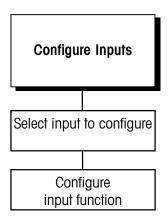
Note: An "OK to Feed" input is required if a FEED prompt will be used. An "OK to Discharge" input is required if a DSCH prompt will be used. Refer to the Memory Program Block for configuring a prompt list.
