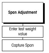
If linearity correction is enabled, you cannot do a span adjustment.
