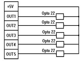
Figure 5-4 Standard Output Wiring
