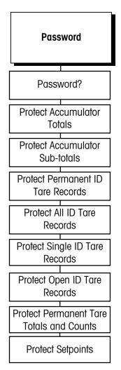
This sub-block lets you create and enable a password that can be used to protect:
