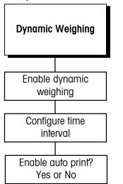
The update rate for an analog load cell system is 20 updates per second. The rate for DigiTOL scales is between 5 and 7 updates per second.
