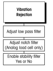
If the scale type is other than analog, the prompt for step 2 does not appear. Begin configuration with step 3. The stability detection feature determines when a no-motion condition exists on the weighing platform. The sensitivity level determines what is considered stable. Printing and tare operations will wait for scale stability before carrying out the command.
