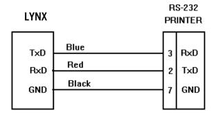
Figure 5-1 RS-232 Printer Cable Wiring
