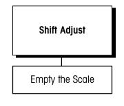
The **Shift Adjust** prompt appears only if you selected Power Module (DigiTOL J-Box) as the scale type. When using a DigiTOL J-Box, each cell's output must be adjusted so that it is equal to the other cells. Cell adjustment is done by applying weight to each cell in sequence as prompted.
