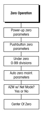
METTLER TOLEDO recommends that power-up zero be disabled by setting Positive and Negative range to 0% for scales such as tanks and hoppers which may lose power in the middle of a control process.
