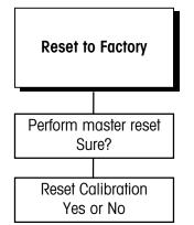
The Reset to Factory sub-block allows you to perform a master reset which returns all parameters for all program blocks to their original settings. To perform a master reset:
