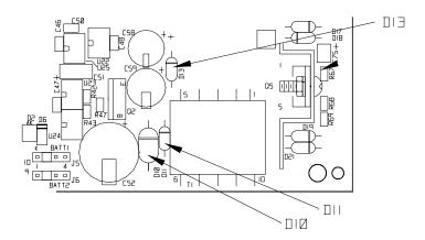
Figure 3-1 Regulated Voltages (on Controller PCB)
