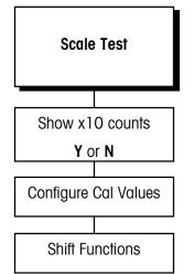
If the scale type is DigiTOL J-Box and linearity correction is enabled, Mid Weight and Mid Counts are displayed. Press **ENTER** to accept the values. This sub-block tests the stability of the scale with regard to the environment and calibration. Scale weight is displayed at a finer resolution than the calibrated increment resolution.
