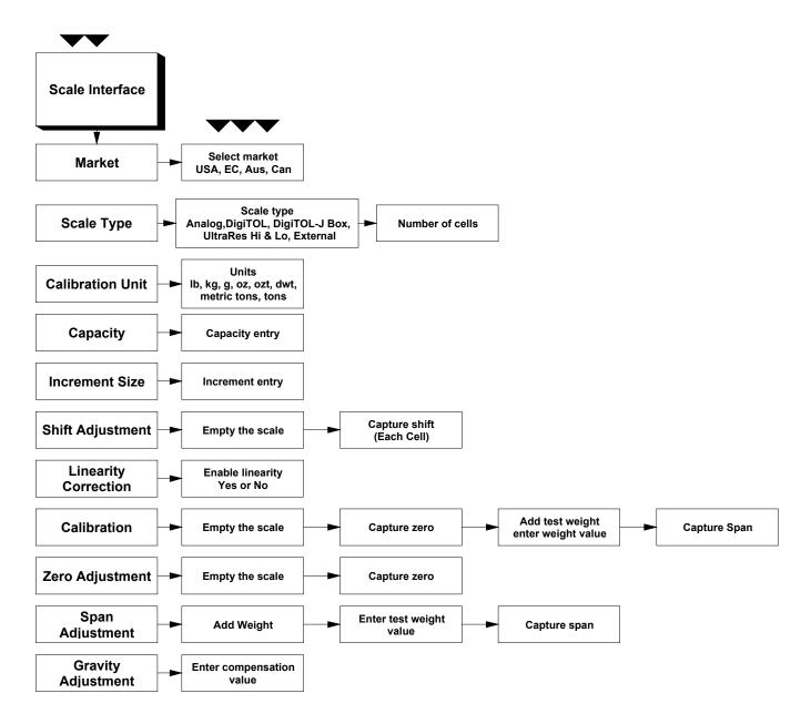
Press **ENTER** at the **Scale I/F** prompt to access the Scale Interface program block and configure the sub-blocks.
