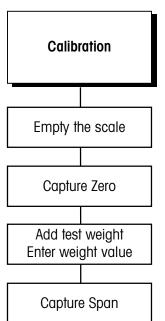
Calibration involves emptying the scale then placing a known test weight on an empty platform and allowing the LYNX terminal to capture values for zero and span. You can calibrate a scale with or without linearity correction. The LYNX terminal prompts you through the calibration.
