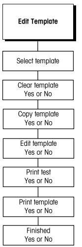
Template ptp03 is used to specify the data format for the last printed data. This data can be uploaded to a host computer using the 8142 host command "Q." Refer to the description in the appendix.
