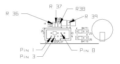
Figure 3-2 Display Voltage Test Points
