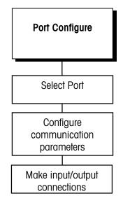
This sub-block lets you configure the serial ports on your terminal for data exchange. You can configure only those ports that are physically available. For example, if a DigiTOL scale is connected, its COM port will not be available for configuration. See Appendix 1 for detailed information on hardware connections, data output format, and template programming and formats.
