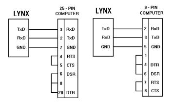
Figure 5-2 Custom Cable Configuration
