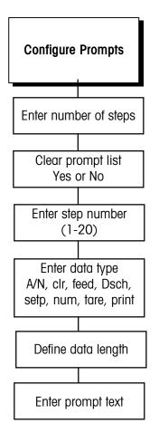
A prompt list displays a written sequence for an operator to perform a task while in Normal Operation mode. You can include up to 20 steps in a prompt list. The LYNX terminal has three preprogrammed prompts:
