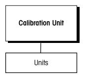
This sub-block lets you enter the units of measure to use when calibrating the scale and configuring capacity and increment size. Recalibration is required if you change the calibration unit.
