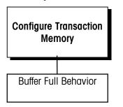
Note that for systems requiring secure data record capture, you should configure this prompt to halt and instruct the operator to notify a designated responsible party if a **Mem Full!** message is displayed. Consecutive numbering is used for sequencing purposes. The LYNX terminal automatically increments the number from a defined starting point. Consecutive numbers can be up to eight digits.
