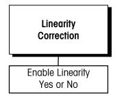
Linearity correction lets you calibrate the scale using calibration reference weights at mid-scale and full-scale ranges. Linearity correction allows for compensation of the non-linear performance of a load cell(s) or weighing system. If linearity correction is enabled, the calibration process requires additional steps. The terminal must be calibrated or recalibrated **after** you enable linearity correction.
